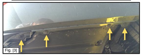
**Step 3.** Remove (3) torx screws from each of the rear wheel wells. Peel back the wheel well liner near the top of the well where the bumper meets the side body panels. Here you will find (1) screw on the driver and passenger sides to remove. See Figure [4], [5], & [6].
