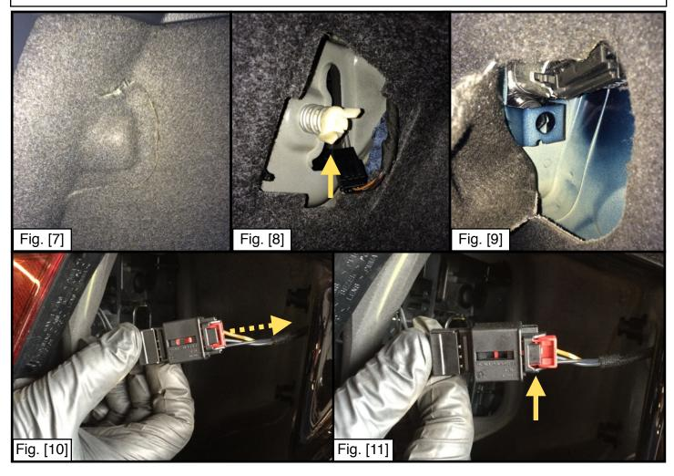
**Step 5.** Starting at the driver side, gently peel the bumper fascia away from the vehicle. Once you reach the tail light section, use a flathead screwdriver or other tool to release the tabs in this section. Move to the passenger side and repeat this process. Unsnap the remaining tabs along the center section of the bumper by pulling rearward. You may need to release the tabs with a flathead in this center section as well. See Figure [12].
