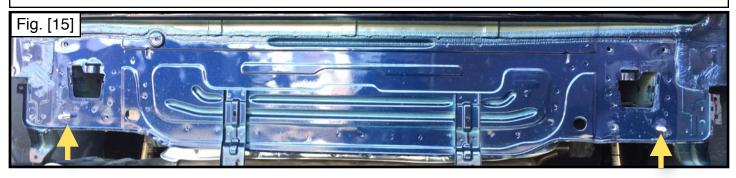
Step 8. Rotate the impact bar into the slot on the left side of the EcoHitch and place the two-piece unit onto the temporary mounting bolts. Secure the hitch and impact bar assembly by threading (1) M8-1.25x40mm Hex Cap Screw, (1) 5/16" lock washer, and (1) 5/16" flat washer through each of the (5) remaining weld nuts and hand tighten. Remove the temporary hanging bolts and install in the same fashion as the other hardware. Torque to 18 ft-lbs. See Figure [16] & [17].
